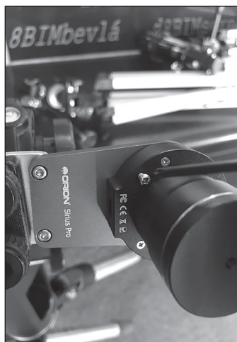
Figure 6. Attach the P1 to the backplate using the three long Philips screws included in the P1 camera box. Note the proper orientation of the connector port -- facing left (towards the mount). The three holes in the camera are through holes (no threads), and the screw threads will engage in the plate behind the camera.
