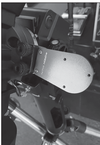
Figure 5. The P1 Sirius Pro back plate fully installed on the Sirius Pro mount
