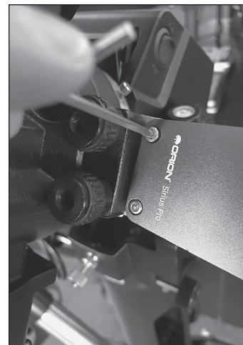
Figure 4. Install the P1 Sirius Pro plate using the socket head cap screws included in the adapter box.
