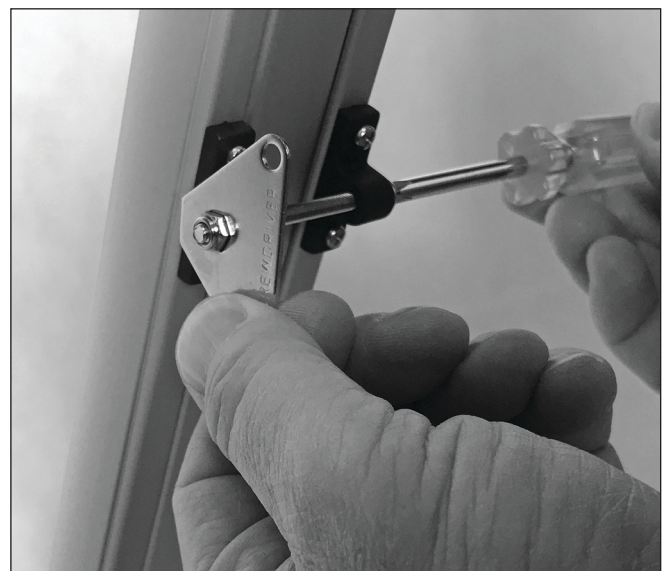
Figure 4. Use the included Philips screwdriver and assembly tool to remove the bracket attachment screw
