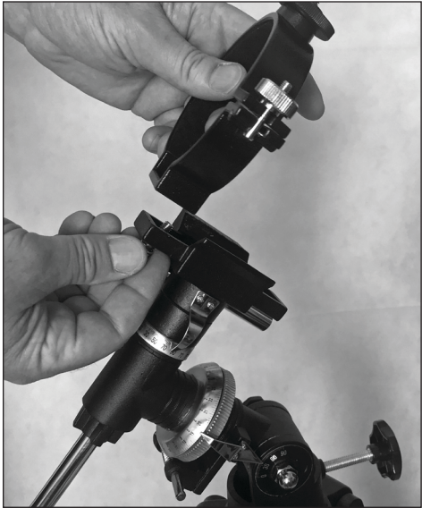
Figure 11. Attach the two tube rings to the equatorial mount's head, making sure the ring with the piggyback adapter on it goes in front.
