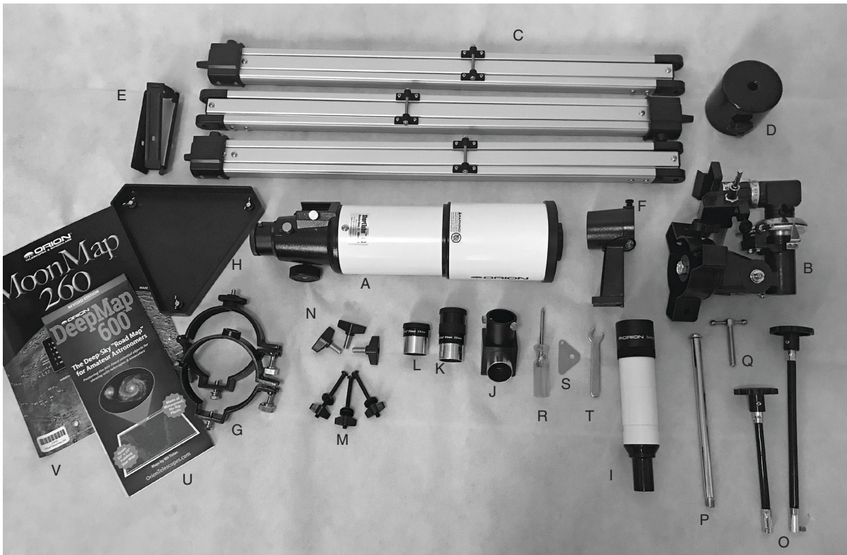
Figure 1. Parts of the ShortTube 80EQ refractor
