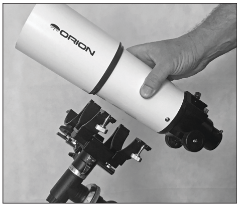
Figure 12. Place the optical tube in the open tube rings, then close the rings and tighten the clamping knobs.
