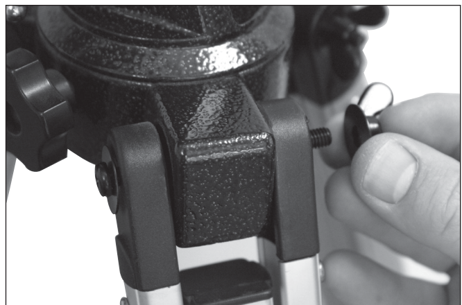
Figure 3. Attaching the tripod legs to the base of the equatorial mount
