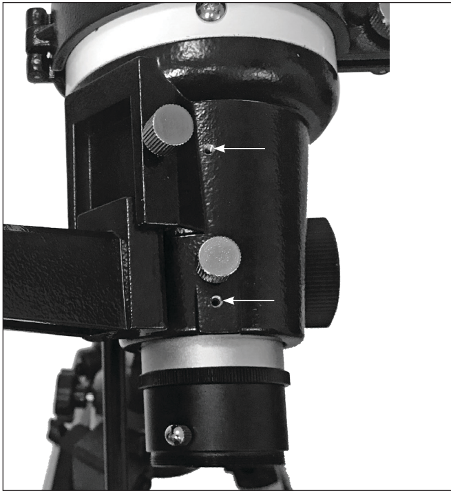
Figure 20. To take out any “play” in the focuser drawtube, use a 1.5mm Allen wrench to lightly tighten the setscrews in the two holes indicated by the arrows.
