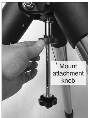
Figure 5. Thread the center post into the mount by turning the mount attachment knob to the right until it is tight.
