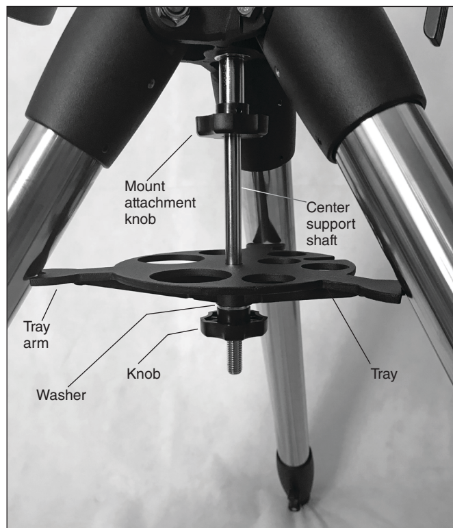
Figure 6. Install the accessory tray, flat side up, as shown. The three tray arms should press against the tripod legs.
