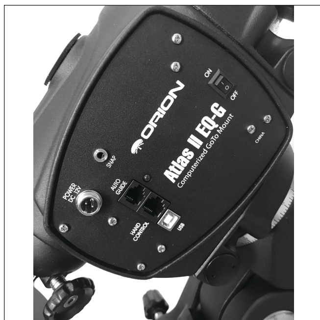
Figure 19. The drive panel of the Atlas II EQ-G
