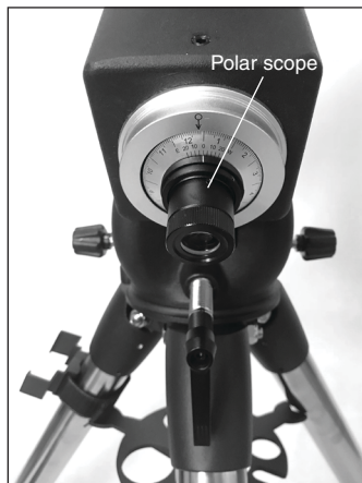
Figure 14. The built-in polar alignment scope works in both the Northern and Southern Hemispheres.
