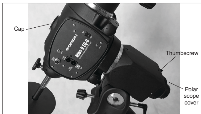
Figure 15. Before polar aligning the mount, you must remove the polar scope cover and the cap on the front of the mount.
