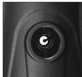
Figure 16. To view through the polar scope, you must rotate the Dec axis of the mount until the hole in the Dec shaft is fully open to transmit light to the polar scope.
