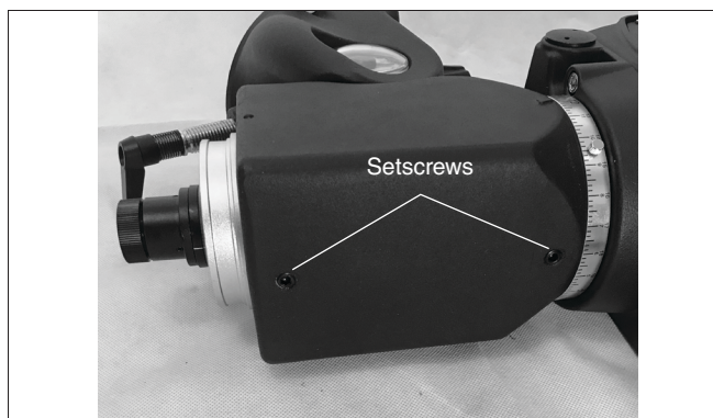
Figure 2. Remove the two setscrews on the mount housing to install the handle.
