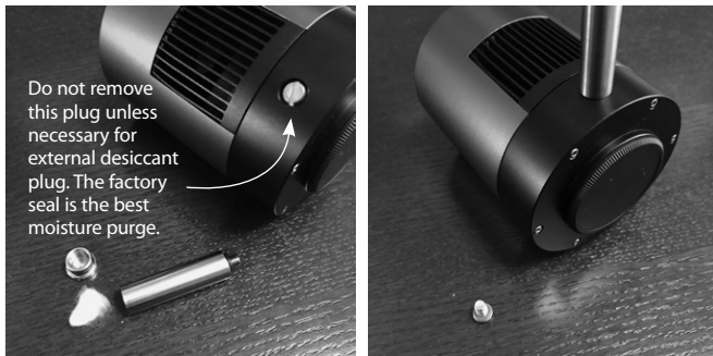
Figure 11a. The desiccant plug. Do not remove the screw plug on the camera body unless you specifically want to use the external desiccant plug. b. The desiccant plug installed in the port. Wait 24 hours for best moisture reduction.
