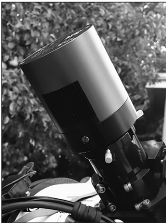
Figure 3a. The Camera, installed in a 2" focuser using the included 2" nozzle
