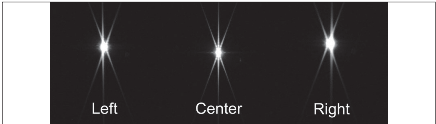
Figure 5. As the telescope's focus is adjusted, the middle spike of the diffraction pattern moves left and right of center of the "X" formed by the other two diffraction spikes. Adjust focus until the middle spike is exactly centered in the X; that's when precise focus has been achieved.
