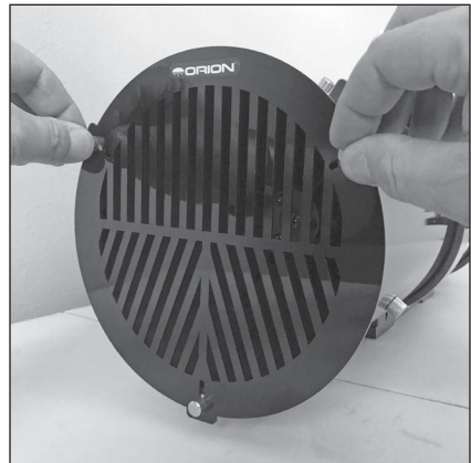
Figure 4. Place the mask over the front of the telescope, then slide the grip posts inward until they contact the telescope's front cell or dew shield before tightening the thumbscrews.
