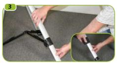
Extend tripod legs 6 to 8 inches by lifting the tripod leg locking lever and pulling the leg to desired length and snapping down the lever.
