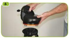
Place the motorized base on top of the tripod making sure that the three round feet rest on the round flat pads on the inside of the tripod head.
