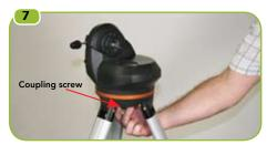
Thread the coupling screw into the hole at the bottom of the motorized base. Tighten screw to secure the base to the tripod.
