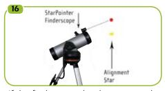
If the finderscope has been properly aligned, the alignment star should now be visible in the field of view of the eyepiece
