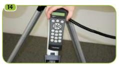
Slide Computerized Hand Control into the hand control holder as shown above.
