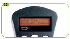
The hand control will display the last entered time and site information. Since this is your first time using the LCM, press UNDO to enter your site and time information.
