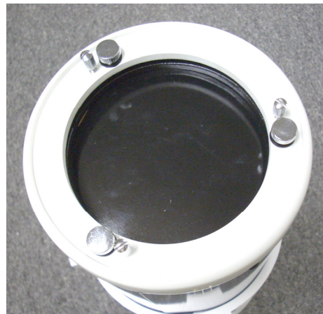
Figure 7-6 Primary mirror. Large thumbscrews are for collimation and small thumbscrews are for locking the mirror in place.
