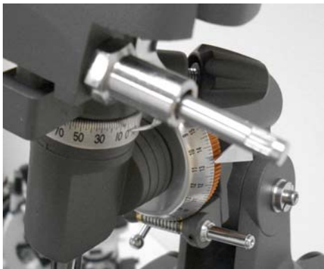
Figure 2-15 R.A. Shaft on bottom and Dec. Shaft on top
