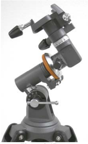
Figure 2-17 Dec. Lock Knob on top of Dec.circle & R.A. Lock Knob on top of R.A. circle
