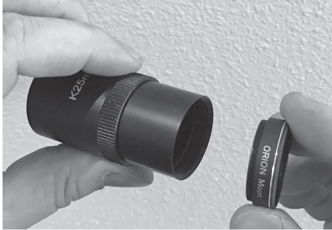
Figure 21. The Kellner eyepieces have barrels threaded to accept optional Orion 1.25" filters. A Moon filter is useful for cutting glare and revealing more detail on the lunar surface.
