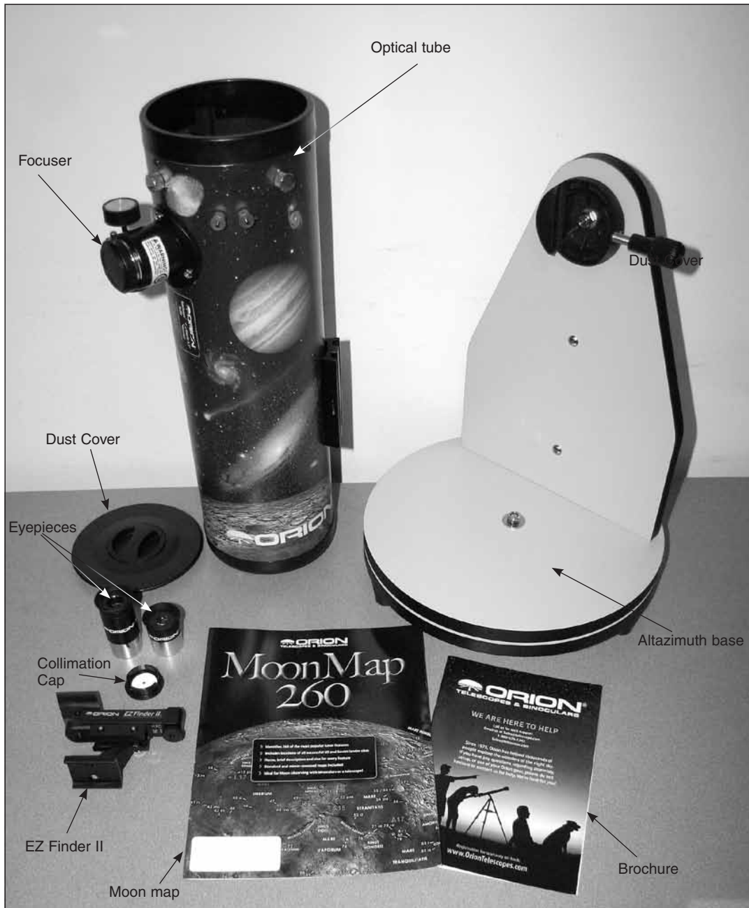
Figure 1. Components of the FunScope Astro Dazzle 4.5. (Not shown: 2mm Allen key and Starry Night digital download coupon)
