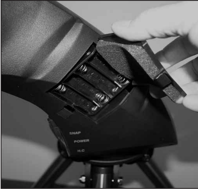
Figure 15. The StarSeeker IV mount is powered by eight user-supplied AA batteries, which are installed in the mount arm.
