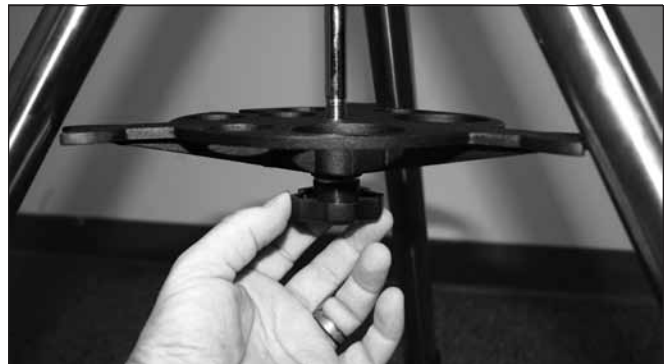
Figure 3. Install the accessory tray/tripod spreader before attaching the mount arm.
