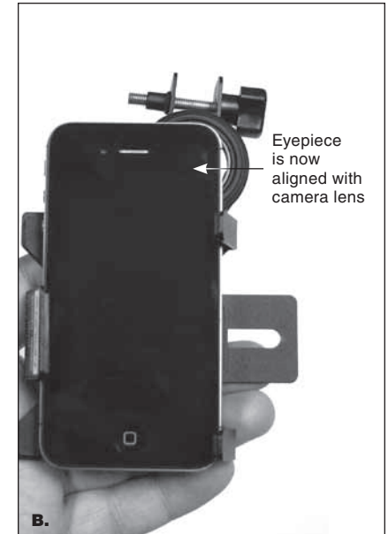
Figure 5. A) The telescope eyepiece is too high to align with the phone's camera. Sliding the phone upward in the bracket allows the eyepiece to align with the camera ( B ).
