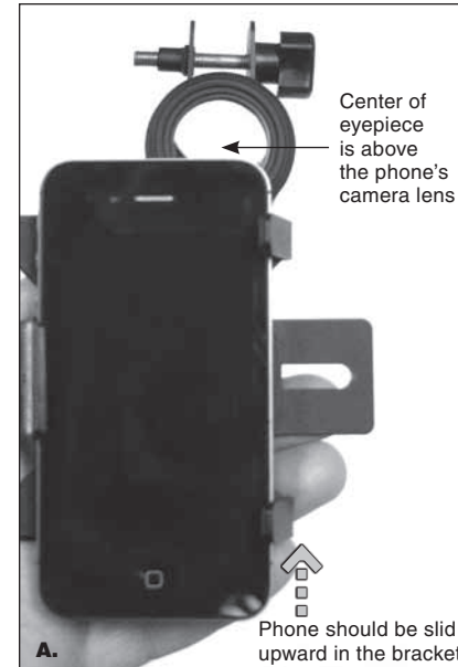
Figure 5. A) The telescope eyepiece is too high to align with the phone's camera. Sliding the phone upward in the bracket allows the eyepiece to align with the camera ( B ).
