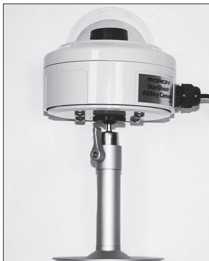
Figure 4. Adapter plate attached to Roof mount bracket.
