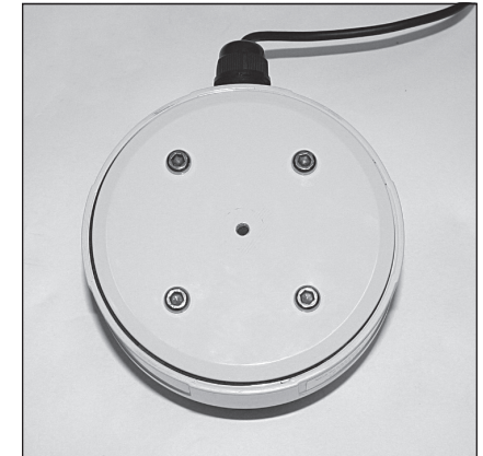
Figure 3. Adapter plate attached to bottom of SASC.
