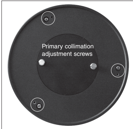
Figure 9. The tilt of the primary mirror is adjusted with three pairs of collimation screws.
