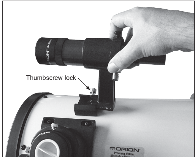
Figure 3. Slide the finder scope bracket into the finder scope dovetail base and secure it in place by tightening the thumbscrew lock.
