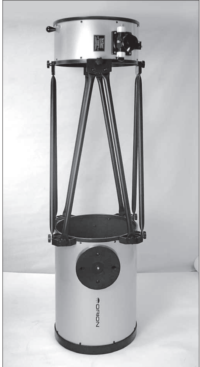
Figure 25. When the optical tube is assembled, the upper tube section should be oriented relative to the lower tube section as shown. Note the orientation of the focuser on the upper tube section relative to the side bearing on the lower tube section.
