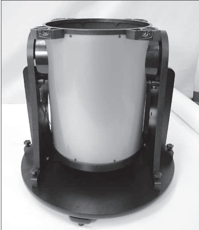
Figure 24. Rather than assembling the entire optical tube and then hoisting it onto the base, some may find it more convenient to mount the lower tube section on the base first, then install the truss tubes and upper tube section.
