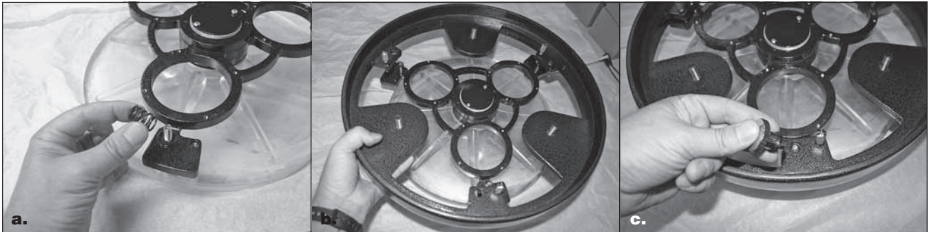
Figure 20. (a) Place the three springs on the exposed threaded shafts of the mirror cell. (b) Lower the rear end ring onto the mirror cell so that the threaded shafts of the mirror cell pass through the end ring, and the end ring rests on the springs. (c) Thread the collimation knobs, with nylon washers attached, through the rear end ring and onto the threaded shafts. Make sure the knobs have at least three full turns of engagement on the shafts.
