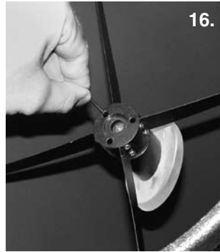
Figure 15. To center the secondary mirror under the focuser, hold the secondary mirror holder in place with your fingers while adjusting the center screw with a Phillips screwdriver. Do not touch the mirror's surface!
