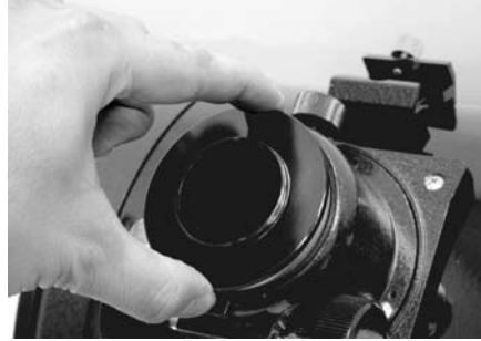
Figure 22b. Thread the camera adapter into the focuser drawtube.
