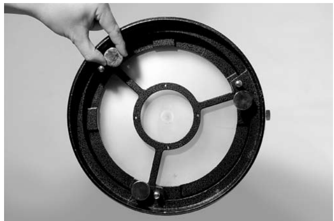
Figure 18. The tilt of the primary mirror is adjusted by turning one or more of the three spring-loaded collimation thumb screws.
