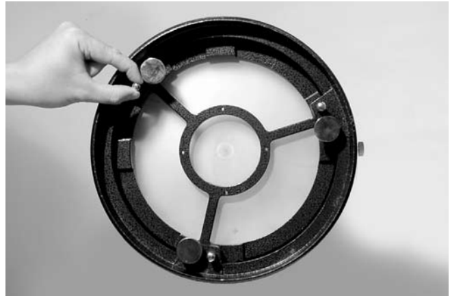
Figure 17. The three thumb screws that lock the primary mirror in place must first be loosened before any adjustments can be made.
