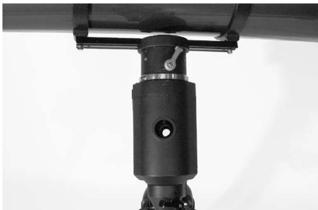
Figure 10. The optical tube must be at a 90° angle to the R.A. axis in order to view through the polar axis finder.
