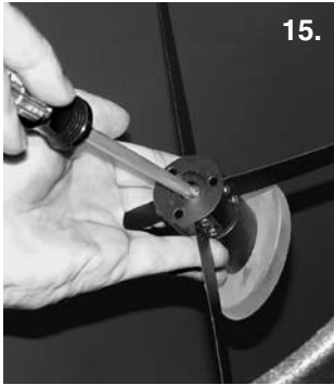
Figure 15. To center the secondary mirror under the focuser, hold the secondary mirror holder in place with your fingers while adjusting the center screw with a Phillips screwdriver. Do not touch the mirror's surface!
