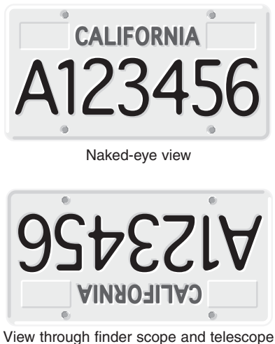
Figure 5. The view through a standard finder scope and reflector telescope is upside down (rotated 180°). This is true for the SpaceProbe 130mm and its finder scope as well.
