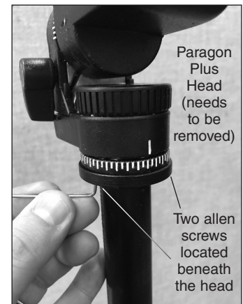
Figure 2. Loosen the two allen screws in order to remove the Paragon Head from the elevator shaft.
