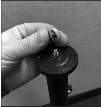
Figure 4. Thread the 3/8"-20 sleeve onto the 1/4"-20 post.
