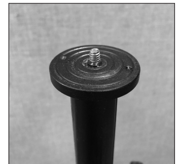
Figure 3. The head has been removed, revealing a 1/4"-20 threaded post.
