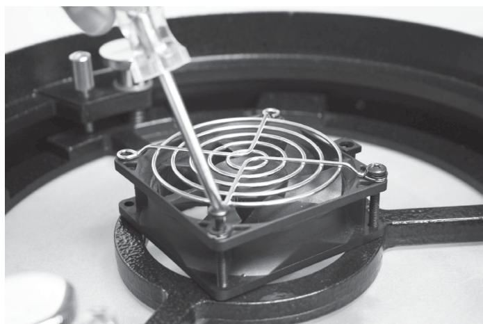
Figure 2. Attaching the fan to the mirror cell.
